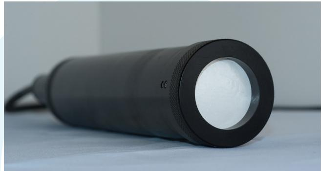
Figure 1. Dissolved CO<sub>2</sub> sensor with membrane equilibrator.
