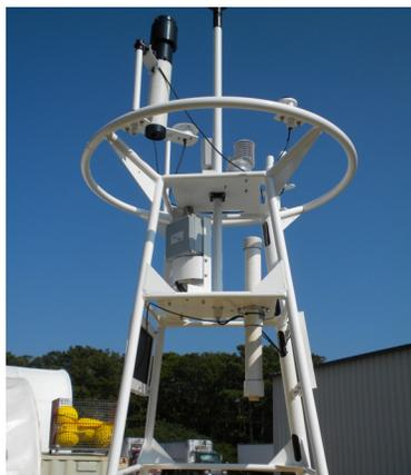
Figure 2. CO<sub>2</sub>-Pro Atmosphere Sensor measures both air and surface water pCO<sub>2</sub> for carbon flux measurements.
