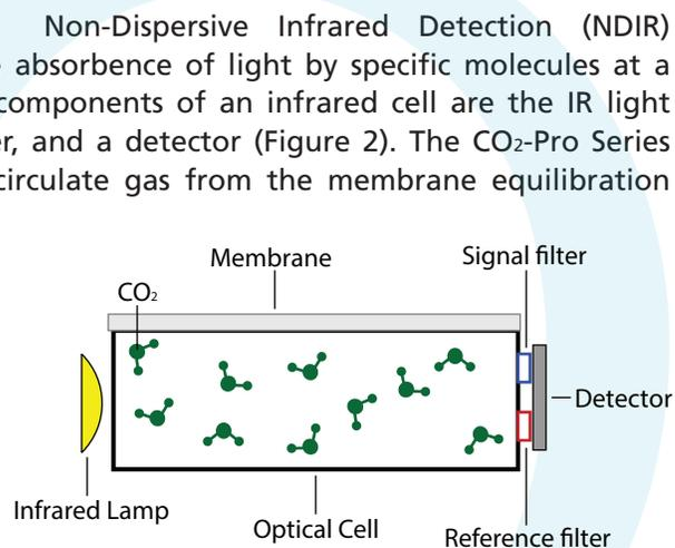
Figure 2. Diagram of infrared detection cell.
