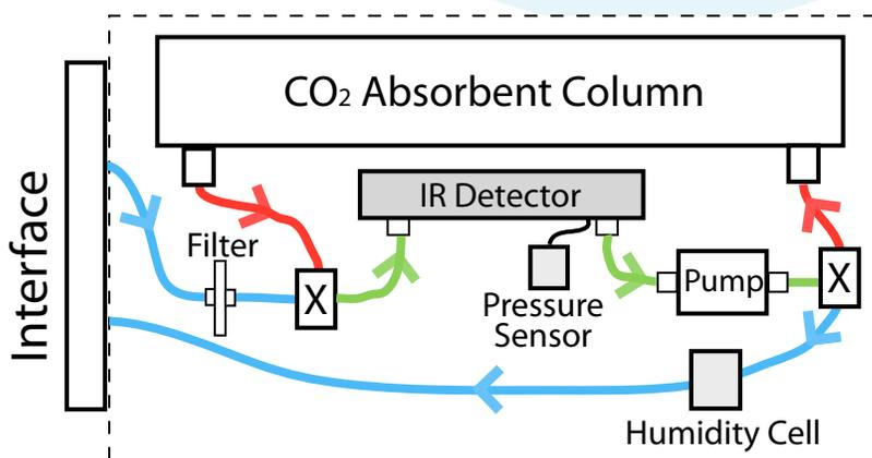
Figure 3. Diagram of the internal plumbing of the CO<sub>2</sub>-Pro Series Instruments.
