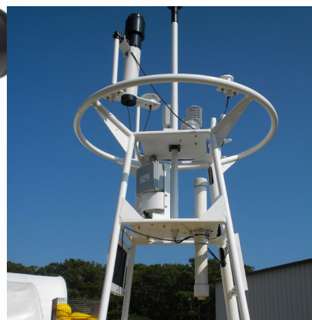
Figure 2. CO 2 -Pro Atmosphere Sensor measures both air and surface water pCO 2 for carbon flux measurements.
