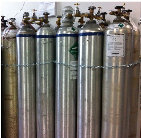
Figure 4. WMO traceable calibration gases.
